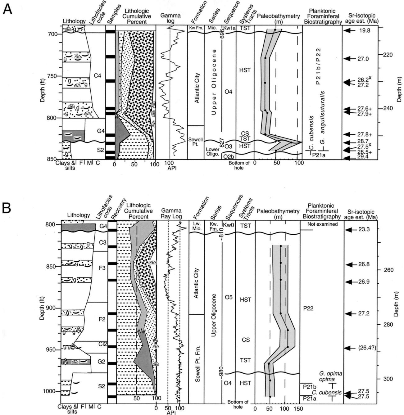
FIG. 5.—Summary diagrams for boreholes at A) AMCOR 6011 and B) Great Bay. See captions to Figures 3 and 4 for additional explanation.
