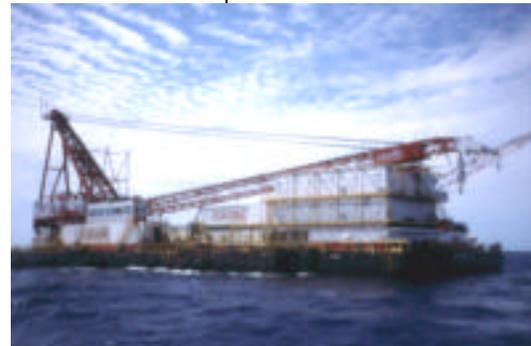
Salvage barge *Wotan* with 500-ton crane used to hoist the *Monitor's* engine in 2001
