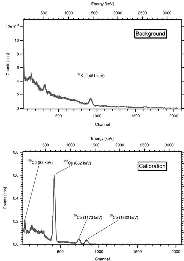
**Figure 3.** (a) Zero-background spectra with the  $^{40}\text{K}$  potassium peak at 1461 keV energy. (b) NGR spectra (counts versus channel) of the calibration standard containing  $^{109}\text{Cd}$ ,  $^{137}\text{Cs}$ , and  $^{60}\text{Co}$ . Total measurement time was 36,000 s. Emission peaks with the corresponding radioisotope and gamma ray energy are indicated. The top horizontal axis shows the calibrated energy scale.
