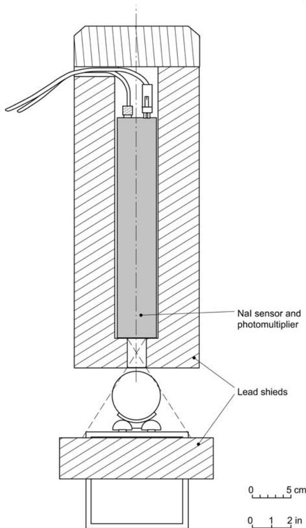
**Figure 2.** Sketch of the geometry of the NGR sensor used on the Rutgers MST.
