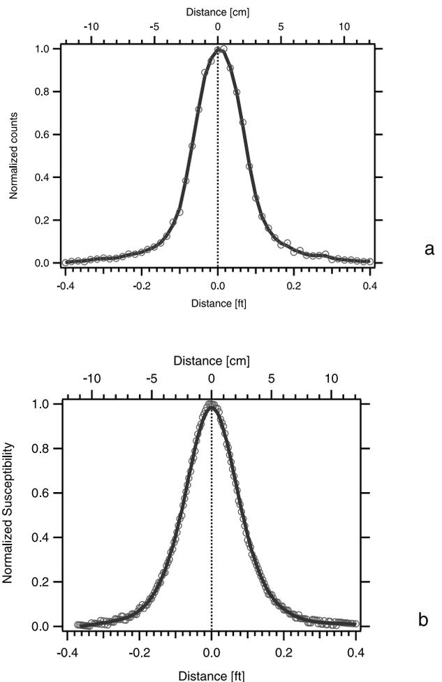
**Figure 4.** (a) Response function  $s$  plotted versus distance from the sensor axis of the NGR sensor using the calibration standard and (b) 100-mm-diameter Bartington susceptibility loop sensor using a thin disk of diabase.
